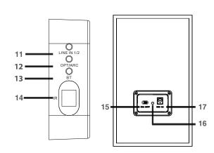
11.[LINE IN 1/2]: Input LINE IN 1LED indicator light (Red lights) / Input LINE IN 2 LED indicator light (Blue lights) 12.[OPT/ARC]: OPTICAL LED indicator light (Red lights) / ARC LED indicator light (Blue lights) 13.[ BT ] : BT LED indicator light (The flashing blue lights) 14.[ IR ] : Infrared remote control receiver 15.[ ON/OFF]Power ON/OFF 16.Connection indicator light(Blue lights)
