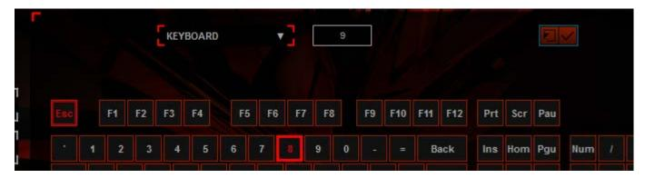
Now drag the 9 key to the 8 key position. The press the red check mark button to confirm this change. As stated above, we have successfully changed the output of the 8 key to 9.
