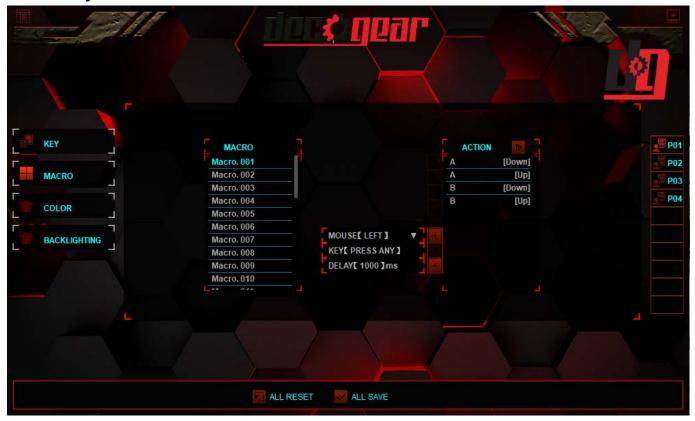
This keyboard supports up to 32 macro profiles. You can switch between any of these saved profiles by clicking the options from the MACRO list on the left, as seen above.
