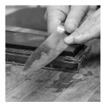
With moderate pressure, slide the blade forward and across the whetstone, covering the entire length of the blade and keeping the blade flush against the stone at a constant 22-degree angle.
